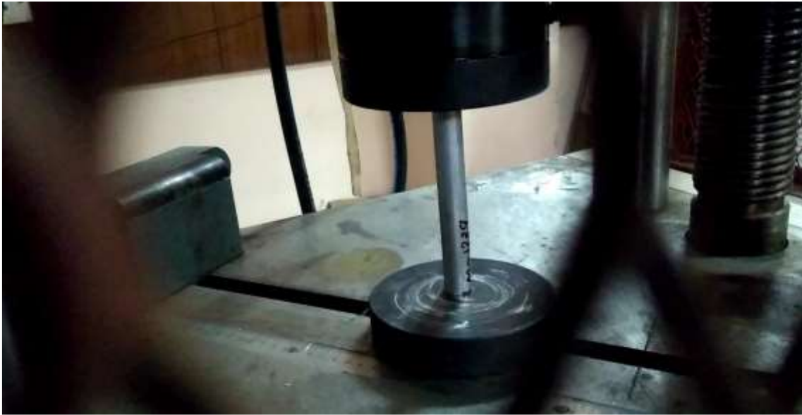
Fig.2. Setup of compressive testing
